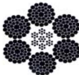
6x49 Filler Wire Seale with IWRC
